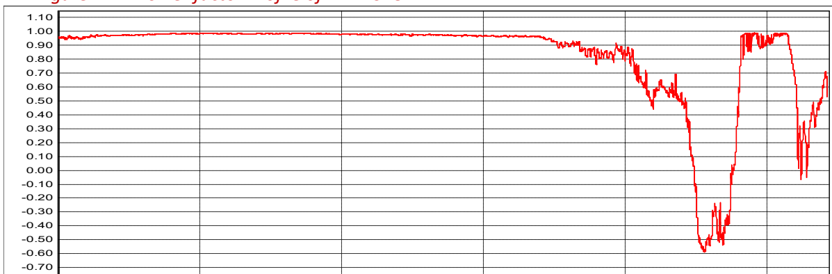
Figure 11. Power factor Profile of TRANSFORMER
